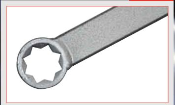
The 1<sup>11</sup>/<sub>16</sub>" Bi-square version of the Industrial Torque Wrench was developed specifically with rail track maintenance in mind. The critical need of the rail industry is to reduce the chance of any object being left on the track. Fitting directly onto rail fishplate bolts means that no socket or square drive is required, two components that could potentially be separated from the regular version of the Industrial Torque Wrench.
